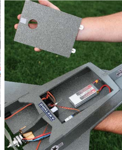
The battery seems lost within the generous equipment bay. With the forward end open, there is tremendous cooling airflow.
